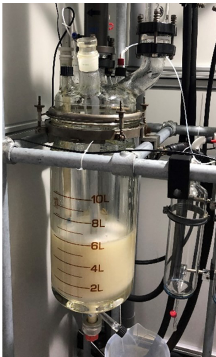
Fig. 1: Enzymatic PET degradation in the 10L reactor
